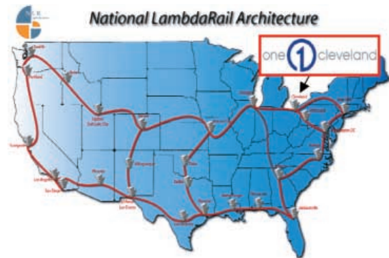
OneCleveland is Ohio’s connection to the National Lambda Rail (NLR), a high-speed network consisting of 10,000 miles of fiber optic cable that connects the nation’s leading research and education institutions.
